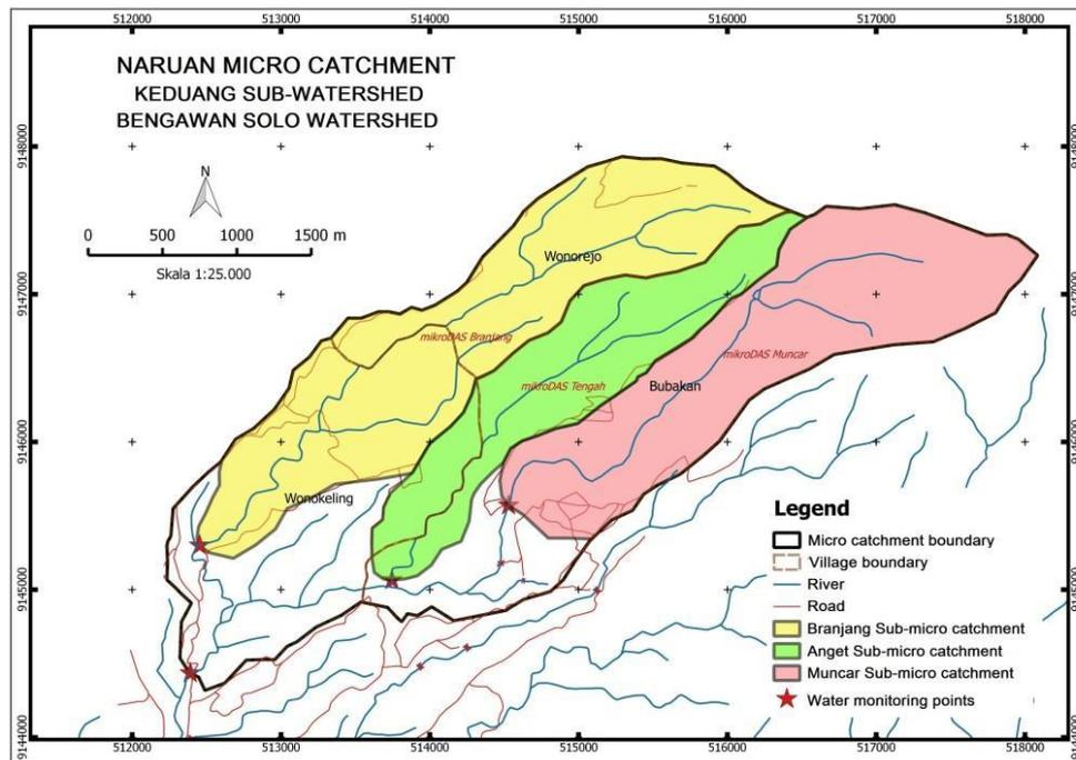
Figure 45. Hydrological monitoring points of NMC
