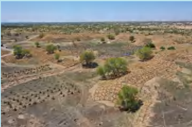
Aerial view of the installed gravel road, sand barriers and newly planted seedlings (@Sanyijing Forest Farm)
